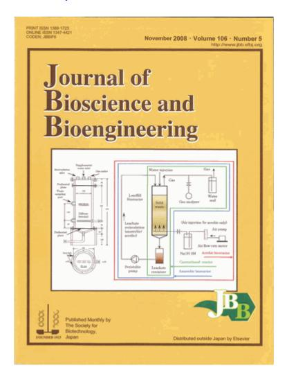
Microbial population dynamics and performance in lab-scale conventional, anaerobic, and aerobic landfill bioreactors specialized for high-organic wastes were investigated. Three acrylic cylindrical bioreactors of 10 cm diameter, 30 cm height, and 2.85 / in total volume were constructed as shown in the figure.
